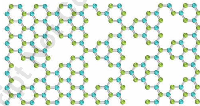
**Fig. 4.** [Reprinted with permission from [9]] Graphene nitride nano sheet, riddled by triangular holes, was experimentally and computationally shown to exhibit an apparent piezoelectric response.
